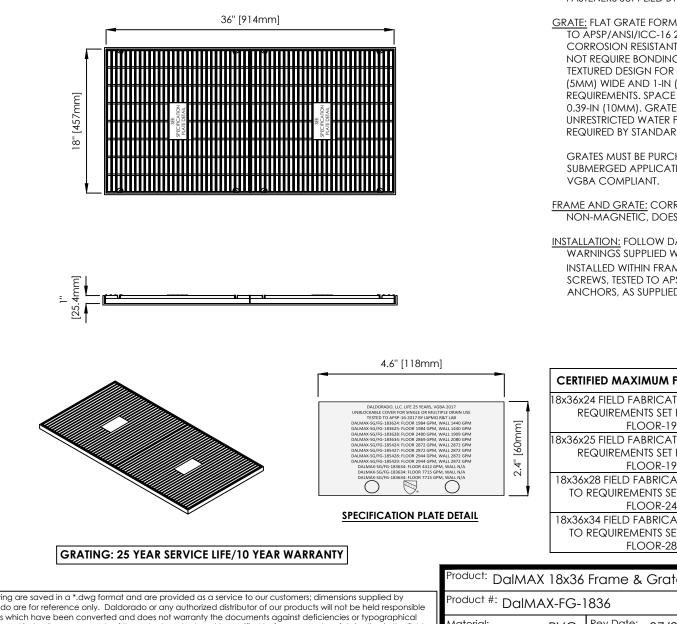
FRAME: CONSTRUCTED OF UV STABILIZED PVC NOTCHED AND HEAT BENT TO SIZE. THE FRAME MUST BE FULLY SUPPORTED AROUND PERIMETER BY MINIMUM 1-IN CONCRETE LEDGE, OR EQUAL, AND INSTALLED USING FASTENERS SUPPLIED BY DALDORADO.
